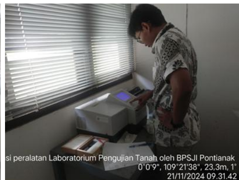
Gambar 12. Proses Kalibrasi In situ Peralatan Laboratorium
